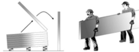
Gripping equipment such as gloves must be clean and such as not to cause damages to the product.
